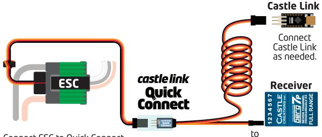
Connect ESC to Quick Connect and leave it plugged in. Use the clear shrink wrap to securely hold the ESC's receiver plug in place. to throttle RX
