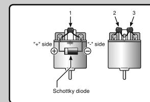
Motors with no suppressor capacitors, or inadequate suppression, may cause the receiver to malfunction. Always solder the capacitors supplied to your motor. The Schottky diode improves the efficiency of the speed control / motor combination and provides extra protection to the brake FETs. The white ring must always face the positive side.
