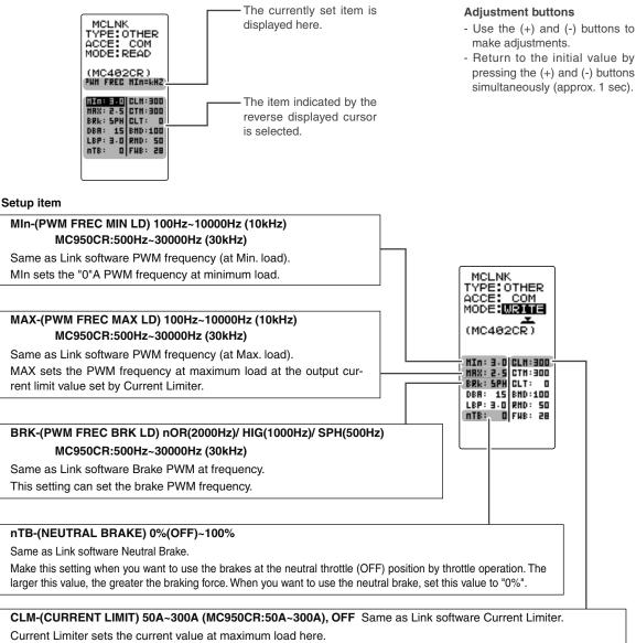
Since setting of the MAX is based on the output current limit value set by Current Limiter, Current Limiter does not have to be turned OFF except when a current exceeding 300A is generated.
