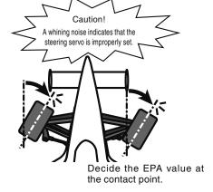
Adjust the steering servo so that unreasonable force is not applied to the servo by the chassis at maximum servo travel.
