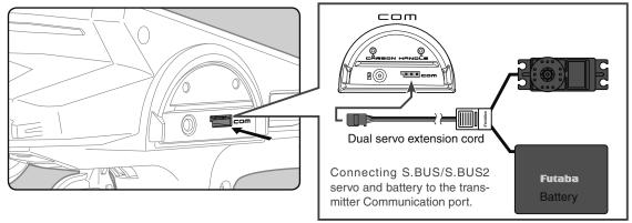
Connection between wireless receiver and servo
