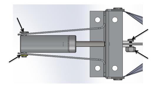
1) Remove cylinder by disassembling retaining clip and pulling out the clevis pin that holds the cylinder to the mounting brackets. Then remove the machine screw and nut that holds the rod end to the retract linkage. The cylinder should drop out freely.
