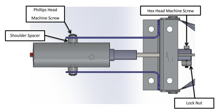
3) With all parts re-assembled as shown above, the conversion is complete.
