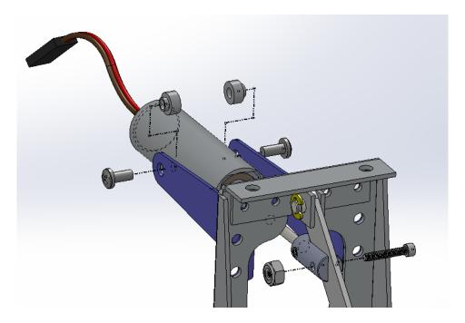
2) Place shoulder spacer with smaller diameter shoulder into the hole in the mounting bracket as shown. Apply threadlocker to screw and thread into actuator housing until tight. Bracket will flex slightly as screws are tightened. Repeat for opposite side. Actuator should be snug but still able to pivot. Thread the cap screw into the aluminum rod end and attach lock nut as shown above. The actuator may need to be threaded in or out by hand to allow for proper alignment.
