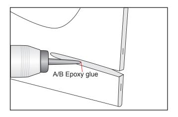
After the epoxy has fully cured, remove the masking tape or T-pins used to hold the stabilizer in place and carefully inspect the glue joints. Use more epoxy to fill in any gaps that may exits that were not filled previously and clean up the excess using a paper towel and rubbing alcohol.
