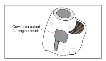
$\Box$  1) Slide the fiberglass cowl over the engine and line up the back edge of the cowl with the marks you made on the fuselage.
