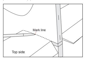
□ 6) Remove the stabilizer. Using a modeling knife and ruler **CAREFULLY** cut 1mm **inside** the marked lines. Remove the covering from the top and the bottom of the tail plane.
