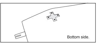
Secure the gear to the wing.
