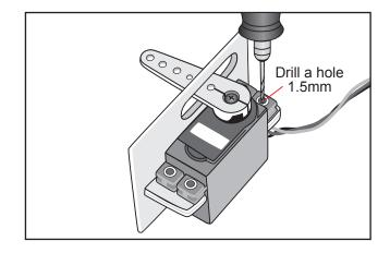
□ 3) Place the servo into the servo tray. Center the servo within the tray and drill 1.5mm pilot holes through the block of wood for each of the four mounting screws provided with the servo.
