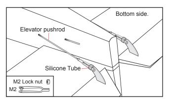
□ 1) Using pliers, carefully make a 90 degree bend down at the mark made. Cut off the excess wire, leaving about 6mm beyond the blend.
