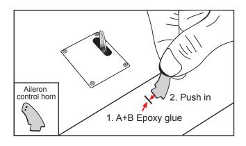
□ 3) Repeat the procedure to install the control horn on the opposite aileron.
