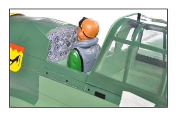
Position the canopy so the rear frame on the canopy is aligned with the rear edge of the cockpit opening. Use canopy glue to secure the canopy to the canopy hatch. Use low-tack tape to hold the canopy in position until the glue fully cures. Wrap the tape completely around the canopy hatch.
