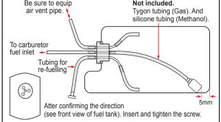
□ 5) Test fit the stopper assembly into the tank. It may be necessary to remove some of the flashing around the tank opening using a modeling knife. If flashing is present, make sure none of it falls into the tank.
