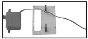
□ 4. Using the thread as a guide and using masking tape, tape the servo lead to the end of the thread: carefully pull the thread out. When you have pulled the servo lead out, remove the masking tape and the servo lead from the thread.
