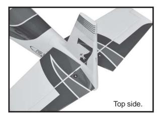
$\Box$  6. Using a modeling knife cut away the covering from the end of fuselage for the rudder hinge.
