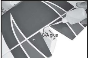
□ 6. After the epoxy has fully cured, remov the masking tape or T-pins used to hold the stabilizer in place and carefully inspect the glue joints. Use more epoxy to fill in any gaps that were not filled previously and clean up the excess using a paper towel and rubbing alcohol.
