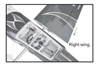
See picture wing attach to fuselage.
