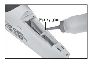
□ 5. When you are sure that everything is aligned correctly, mix up a generous amount of 30 minute epoxy. Apply a thin layer to the top and bottom of the stabilizer mounting area and to the stabilizer mounting platform sides in the fuselage. Slide the stabilizer in place and re-align. Double check all of your measurements one more time before the
