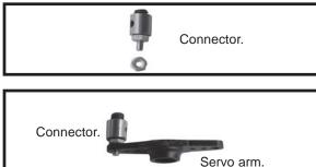
After installing the adjustable metal connector apply a small drop of thin C/A to the bottom nut. This will prevent the connector from loosening during flight.
