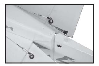
$\square$  3. Secure the tail wheel bracket in place using three 3mm x 12mm wood screws. Be careful not to overtighten the screws.
