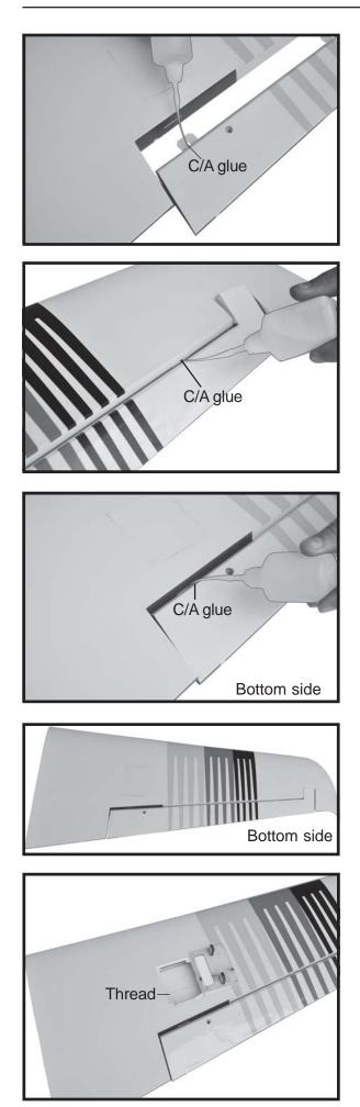
□ 2. Using a modeling knife, remove the covering servo tray.
