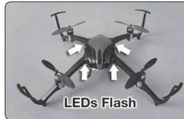
2. Slide the flight battery into the slot on the underside of the Verso. Connect the flight battery to the Verso and place it upright on a level surface. The LEDs on the quad will flash rapidly while the quad is linking to the controller. Then they will blink slowly while it waits for the arming routine.
