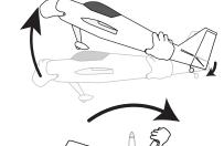
Tilt the airplane to the left on the ground and check that the rudder operate to the right. (In the case of rudder control)
