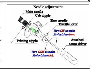
Suppose the peak speed with the tank filled full with fuel is at 9,500rpm, set the main needle to reduce the peak speed by 300 rpm at 9,200rpm. Run the engine at a speed about 300rpm lower than the peak to prolong the service life of the engine and minimize rusting on bearings.
