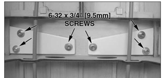
❑ 5. Insert the landing gear legs into the slots in the fuselage. Attach the gear to the fuselage using six 6-32 x 3/4" [19mm] SHCS, six #6 flat washers, six #6 lock washers, and threadlocking compound.
