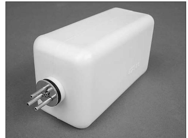
❑ 2. Fit the stopper assembly into the tank with the vent line pointing toward the top of the tank, but not touching. The fuel tubing and clunks (fuel pickup) on the carb and fill lines should almost reach the back of the tank but not touch. The clunks must be able to move freely inside the tank when assembled.
