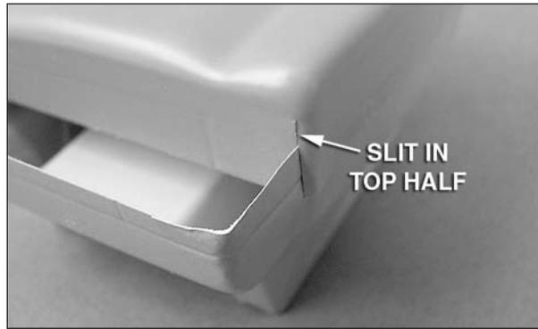
❑ 2. Begin by cutting out the seat bottoms for the front seats. Canopy scissors work well for this. There are cut lines on the parts. However, we suggest cutting approximately 1/4" [6mm] beyond the cut lines and assembling the halves by overlapping the edges. (If you choose, you could cut along the cut lines and edge glue the two halves together. Because the pieces come pre-painted, a good fit would be difficult doing it this way). Small slits will need to be
