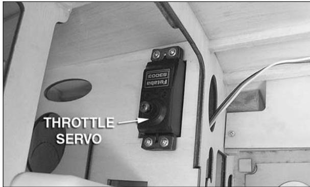
❑ 7. Install the throttle servo in the location shown. Because of the tight working space here, a Hobbico Pin Vise (HCAR0696) is very useful in this step. Use the hardware included with the servo.
