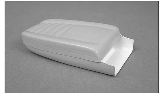
❑ 3. The seat back halves are cut and assembled the same way. Make note how the bottom edge of the seat back is trimmed to fit inside the seat bottom. This is a trial and error fit, so trim away small amounts at a time and test fit the piece until a good fit is achieved. When satisfied with the fit, finish sand the edges and glue the halves together.
