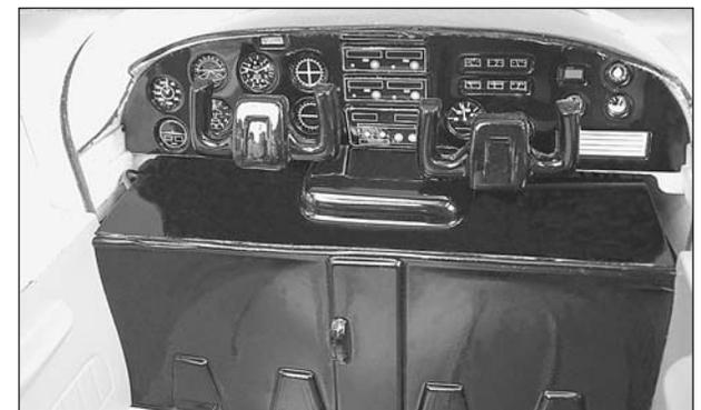
❑ 10. Glue the steering yoke dowel rods into the recesses in the instrument panel. Test fit the instrument
