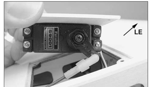
3. Slide the pushrod through the access hole in the wing and connect the bent end of the pushrod to the outer hole in the flap control horn using a nylon FasLink. Connect the clevis to the outer hole in the flap servo arm. Put the flap servo hatch cover in place onto the wing. While holding the hatch cover down, use your radio system to test the operation of the flap. Make any adjustments necessary to the position of the clevis on the pushrod or the servo arm.
