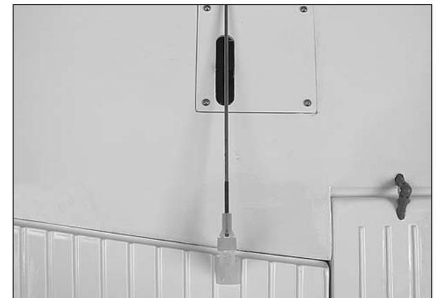
8. Position the control horn onto the aileron between the two corrugations that are inline with the aileron servo arm. Align the holes in the control
