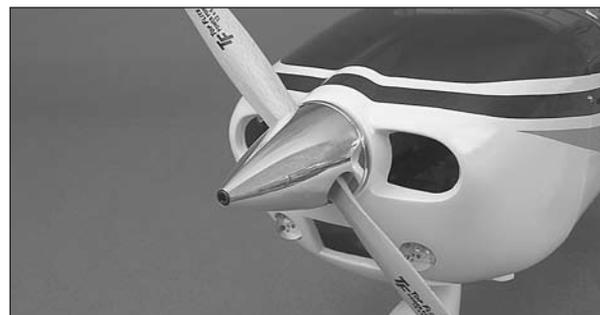
□ 3. Tighten the spinner cone to the backplate using the 4 x 45mm SHCS.
