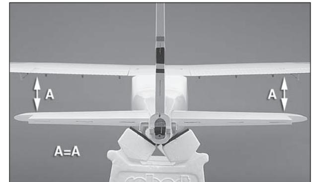
❑ 1. Temporarily attach the wing to the **fuselage** using two 1/4-20 nylon wing bolts. The nylon wing dowels fit into receiving holes in the former just behind the location of the windshield. Test fit the **horizontal stabilizer** into the saddle in the fuselage. The beveled TE on the stab should slope forward from the top of the stab to the bottom. If not, the stab is installed
