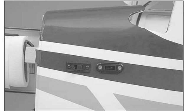
❑ 6. Install your receiver switch and charge jack on the side of your fuselage. Be sure that the location you choose will not interfere with servos, pushrods, or the cockpit (look ahead in the manual to see the position of the cockpit kit components).
