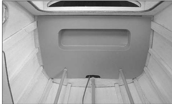
❑ 6. Cut out the cockpit back panel. Slots will need to be made for the elevator and rudder pushrod tubes, as well as a cutout for the tail light wire to pass under. The piece should sit flat against the fuselage former just behind the back window. Glue the cockpit back in place. *Work slowly during step 7 to cut cockpit side panels that fit well.*
