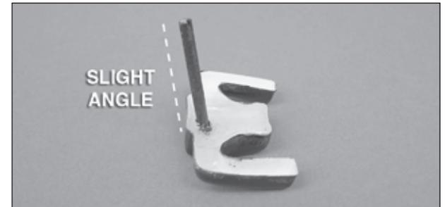
❑ 9. Cut out the steering yokes and sand the bottom edges smooth. Fill the inside center of the yokes with epoxy and embed the included 1/8" x 1-1/2" [3 x 38mm] dowel rods into the epoxy. Set them at a slight angle as shown. Just as the epoxy begins to get hot and harden, hold the dowels in the desired position while the epoxy finishes hardening.
