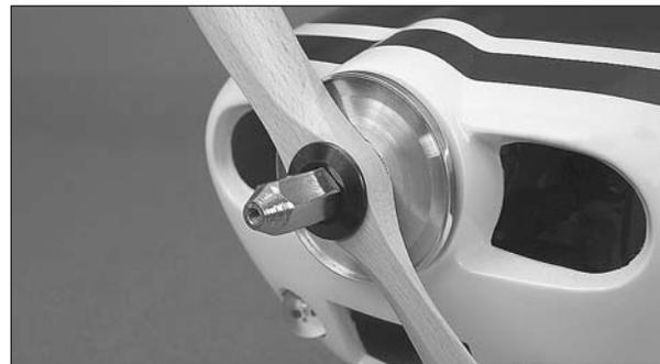
□ 2. Ream your prop as necessary. Install the spinner backplate, propeller, propeller washer and spinner nut onto the engine crankshaft. If you installed a four-stroke engine, use the four-stroke spinner nut.
