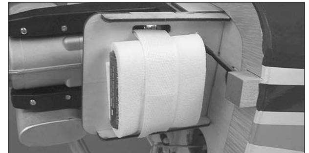
❑ 1. Make a hook and loop strap for your receiver pack from the included hook and loop material by overlapping mating ends by approximately 1" [25mm]. The total length of the strap will depend on the size of your battery. Wrap the pack in foam rubber (not included) and use the strap to secure it to the side of the motor mounting box as shown.
