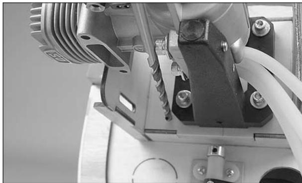
❑ 8. Drill a 3/16" [4.8mm] hole in the firewall inline with the throttle arm on the carburetor at a slight angle pointing to the throttle servo. We used an extra long drill bit (HIGR1020). If you do not have an extra long bit, you may need to mark the location for the hole on the firewall and temporarily remove the engine to drill the hole. **Make sure you do not drill into the fuel tank!**
