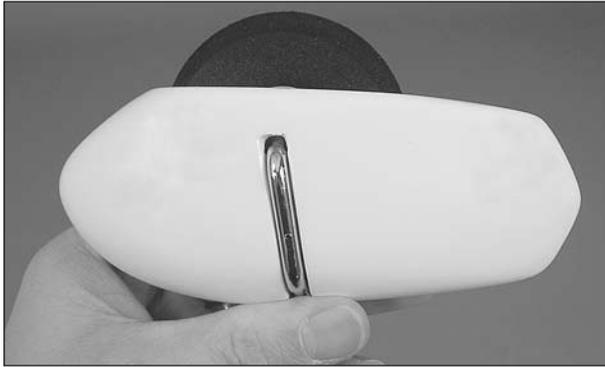
❑ 6. Insert the nose gear wire into the front wheel part as shown. Slide a 5.5mm wheel collar onto the nose gear wire followed by the 2-3/4" [70mm] nose wheel, and another 5.5mm wheel collar. Center the wheel in the pant and mark the location of the wheel collars onto the nose gear axle. As you did with the main landing gear, file flat spots at the marks you made.
