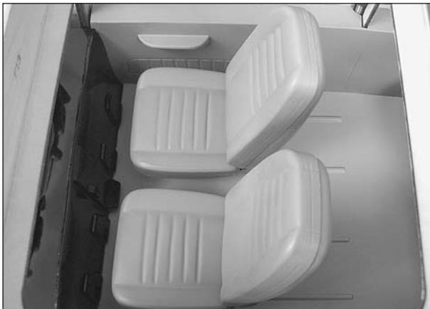
□ 11. Glue the seats to the cockpit floor. Remember, the seats should also be removable in case the floor needs to be taken out. Hot glue works well for this. Small dots of medium or thick CA could also be used.
