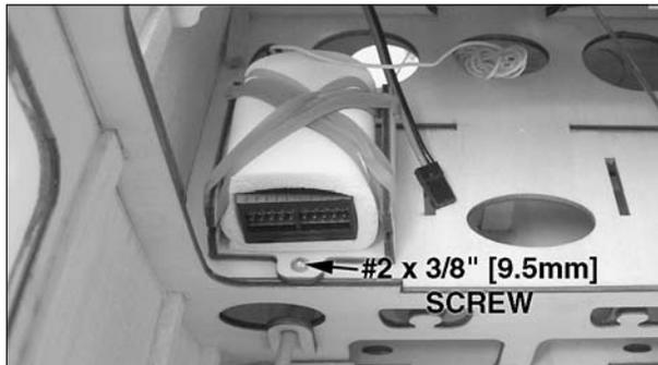
❑ 5. Slide the tab on the underside of the receiver tray onto the forward edge of the unused throttle servo
