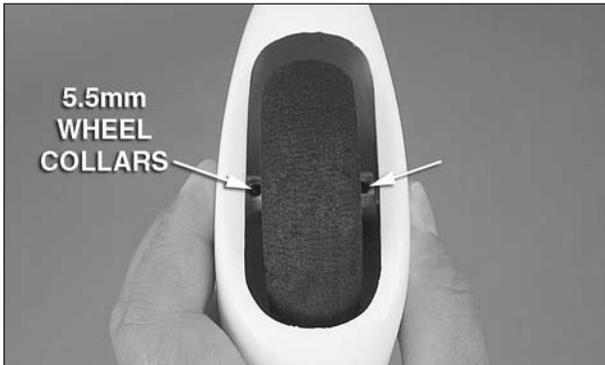
❑ 7. Loosely thread a 3 x 4mm machine screw with threadlocking compound into each 5.5mm wheel collar. Reinstall the wheel collars and nose wheel onto the nose gear wire along with the wheel pant. Tighten the screws in the wheel collars onto the flat spots you made on the axle. Confirm that the wheel spins freely on the axle. Add oil as necessary.
