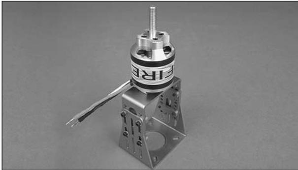
❑ 1. Attach the motor to the brushless motor mount using four 3 x 8mm machine screws, four 3mm flat washers, and threadlocking compound. You may need to remove the brass collar to fit the motor to the mount. Be sure and replace the collar after the motor is installed. If you haven't done so already, install the prop adapter to the front of the motor using the hardware included with the motor and threadlocking compound.
