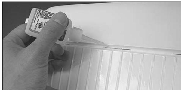
❑ 3. Fit a CA hinge into each hinge slot in the stab. If the hinges are difficult to install, use a hobby knife to slightly enlarge the slots. Roughen the ends of the
