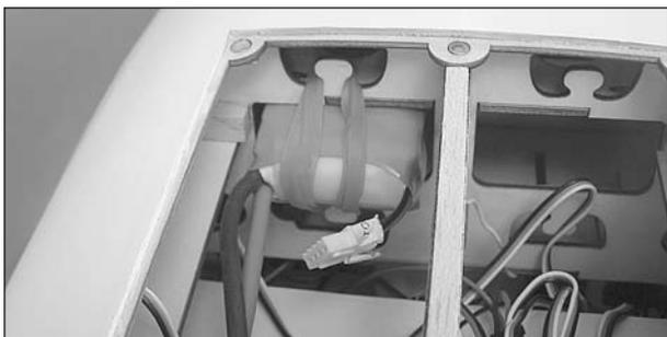
❑ 5. LiPo battery compartments are located inside the battery hatch. Since the recommended battery
