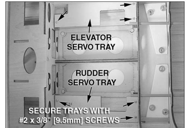
❑ 1. Position the **elevator** and **rudder servo trays** onto the hardwood rails glued inside the fuselage as shown. Drill through the mounting holes in the trays into the
