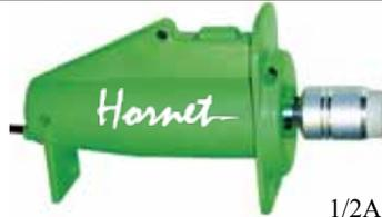
**Hornet.** Designed for small, high RPM engines, such as 1/2A and control line. 12 Volts with a maximum of 30 Amps. 15,000 no load RPM. For all engines up to .12 cubic inches (2.0 cc). No. S598
