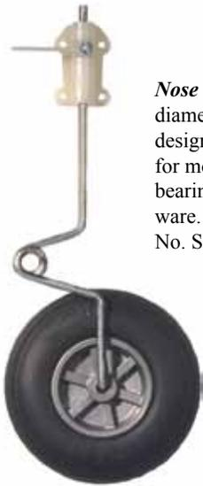
**Nose Gear.** Made from plated 5/32" diameter music wire. Special "knuckle" design absorbs shocks. Extended leg for more adjustment range. Includes bearing block, steering arm and hardware. Tire not included. No. S865
