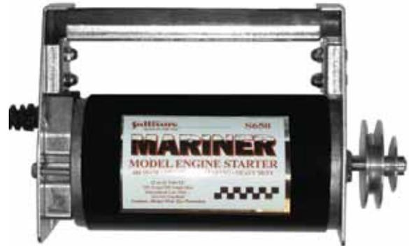
**Mariner.** Heavy duty starter made for starting boat engines with starter belts. Top handle with switch. Aluminum Double Pulley Drive Cone. 12 or 24 Volts with a maximum of 100 Amps. 600 in-oz of torque on 12 Volts, 1200 in-oz on 24 Volts. 2800 no load RPM. No. S650
