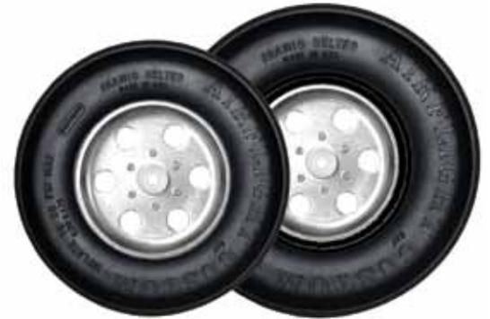
**"SkyLite" Large Scale Light Weight Wheels with Aluminum Hubs.** Two-piece removable aluminum hubs have a Delrin center bearing. Hubs include pockets for optional ball bearing. Tires are scale in shape, tread design and lettering.
