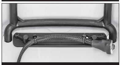
Rear Light Bar Wiring/Long Extension Harness installed on Rear Light Bar Mount
