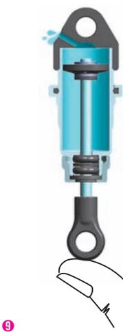
**9** Gently push the shock shaft completely into the shock body. Excess oil will flow through the hole in the shock cap.
