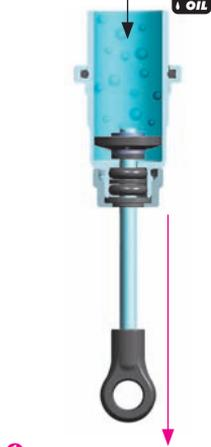
**1** Extend the shock shaft completely. Fill the shock body with the shock oil. For the FRONT shocks (short) use 450cSt oil. For the REAR shocks (long) use 400cSt oil.
