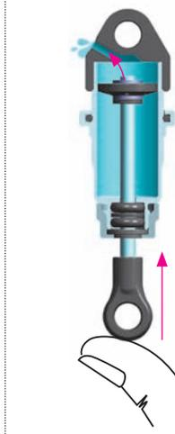
**5** Gently push the shock shaft completely into the shock body. Excess oil will flow through the hole in the shock cap.
