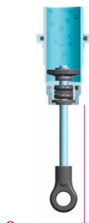
**3** Orient the filled shock vertically for several minutes with the shock shaft fully extended. The remaining air bubbles will release.
