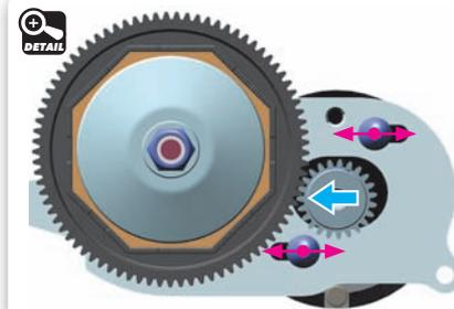
Adjust the motor so the pinion meshes with the spur gear properly. Make sure the gear mesh is not too tight.
