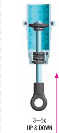
**2** Move the shock shaft up and down a few times to release the air bubbles trapped beneath the piston.
