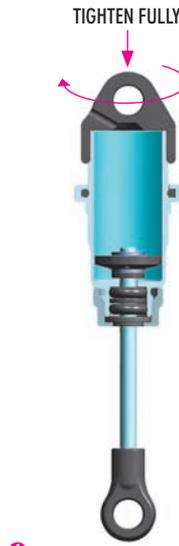
**4** Gently place the shock cap onto the filled shock body and start to tighten the cup. Tighten the cap fully.
