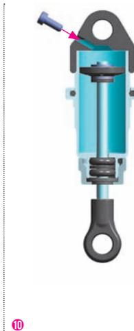
**10** Tighten the screw. The rebound will be at approx. 0%
