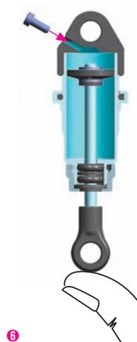
**6** Keep the shock shaft pushed in the shock body and insert the screw into the shock cap. Tighten gently.
