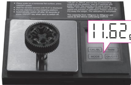
1 Put the diff (without oil) on the scale and check the weight (approximately 11.62g)
