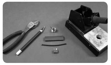
1 female Deans<sup>®</sup> connector 1 short length of 12 or 14 gauge wire 1 length of large shrink tubing Soldering Iron (TrakPower<sup>™</sup> TK950, TKPR0950) Solder, (TrakPower Lead Free Solder, TKPR0975) Hobby knife Wire cutters Lighter or heat gun
