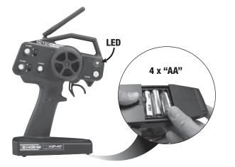
**1.** If you have the Performance 2.4GHz version, install 4 "AA" batteries into the transmitter using the installation pattern molded into the bottom of the battery tray. Turn on the transmitter, making sure it's working by viewing the LED on the front. The LED should glow bright red.
