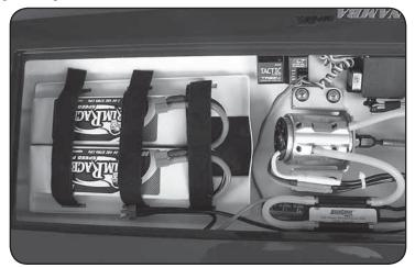
**2.** Remove the canopy and install the batteries, making sure they are well strapped in and seated.
