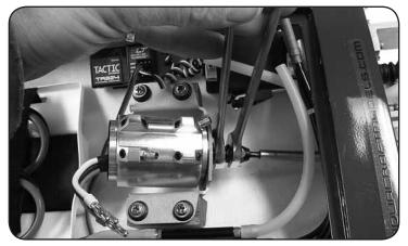
**2.** Use the 12mm and 10mm wrenches to loosen the cable coupler from the cable. To do so hold the 12mm wrench still and rotate the 10mm wrench counterclockwise.
