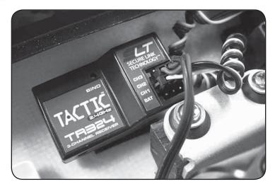
**2.** Plug the steering servo into channel 1 and the motor controller into channel 2.
