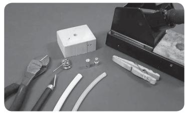
5.5mm Bullet connectors (Castle Creations, CSEH0002) Soldering Iron, (TrakPower TK950, TKPR0950) Solder, (TrakPower Lead Free Solder, TKPR0975) Hobby knife Wire cutters Shrink tubing (yellow) 6" length of large fuel tubing Lighter or heat gun
