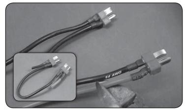
**1.** One inch from the connector cut both the black and red wires leading from the controller. Do not cut the black jumper wire between the connectors. Set this part aside as it can be used to make an adaptor if you solder corresponding bullets to the cut wires.
