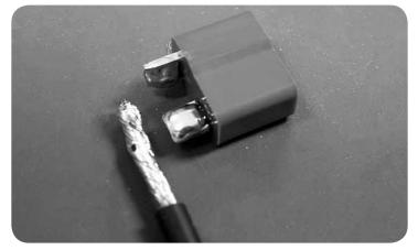
**1.** Begin by tinning (pre-applying) solder to both the positive and negative solder tabs on the Deans connector; also remove about 3/4" of insulation off one end of the length of wire and tin the exposed wire as well.
