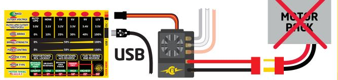
Field Link and ESC are both powered by the USB connection
