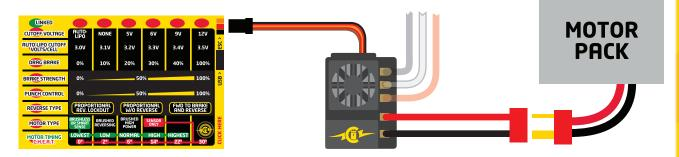
Field Link and ESC are both powered by the motor pack
