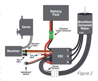
to change the motor direction, use Castle Link, manually programming or B-Link Adapter.
