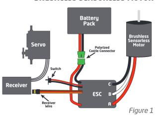
If you choose to direct solder or to shorten the motor wires, you may do so on the Castle Creations 14XX series, 15XX series, 1717, and 2028 motors only. DO NOT CUT any part of the wire length from any other motor, regardless of brand or type. In most cases, only the last 1/4 inch or so of the motor wires are able to be soldered. If they are clipped shorter you may not be able to solder the remaining portion of the wire and the motor will not run properly, if at all.
