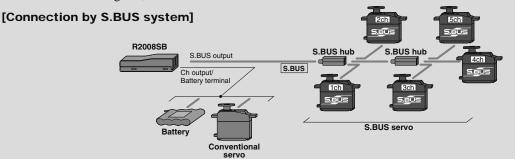
\* Set the channel at the S.BUS servos by using an SBC-1 channel changer or a CIU-2 USB serial interface.
