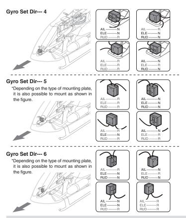
It is necessary to set the motion direction of each gyro by "AGy.Dir", "EGy. Dir" of "SWH. BASIC" menu (page 50) and "Gyro.Dir" of "RUD BASIC" menu (page 58).
