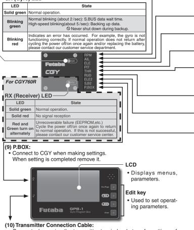
• Connect when using the transmitter to wirelessly transfer settings of GPB-1 to CGY.
