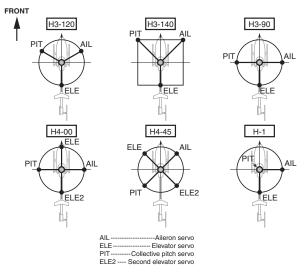
Your transmitter should be reset to the default settings and the swash plate type selected with the transmitter should be set to "H-1" or single servo mode. All CCPM mixing is set up and handled in the CGY, and the transmitter functions should not be used. Before starting model set-up, be sure that all dual rates, pitch curve, and endpoint values are set to 100/100.
