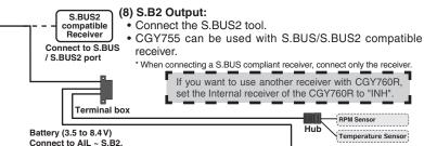
(Never connect to RPM and P. BOX connector)
