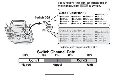
If you set a condition switch channel, using the AFR function on that channel set a flat point curve for each flight condition. Then you can utilize all 5 flights conditions.
