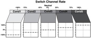
Set the point curve with AFR for each flight condition of the transmitter.
