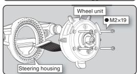
**7** Pass the wiring from the wheel unit through the hole in the APA parts and steering housing as shown in the figure.
