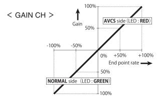
3CH (GAIN CH) is set up with reference to the manual of a transmitter. A neutral becomes GAIN 0%. It is divided into AVCS side and NORMAL side. Check using the GYC430's LED.
