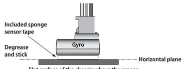
Flat surface of the chassis where the sensor tape sticks easily. Mount the gyro level so that it is not tilted relative to the chassis.
