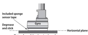
Flat surface of the chassis where the sensor tape sticks easily. Mount the gyro level so that it is not tilted relative to the chassis.
