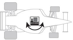
The direction of rotation fixed by the gyro can be any direction within 360° relative to the steering axis controlled by the gyro.
