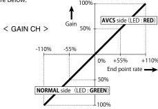
3CH (GAIN CH) is set up with reference to the manual of a transmitter. Neutral position becomes GAIN 0%. It is divided into AVCS side and NORMAL side. Check using the GYD470's LED.
