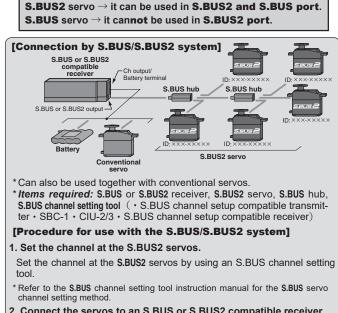
Connect the servos to an S.BUS or S.BUS2 compatible receiver. Connect the servos from the S.BUS or S.BUS2 port of the S.BUS or S.BUS2 compatible receiver via S.BUS hubs.
