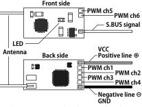
When using S.BUS, solder the S.BUS line of S.BUS equipment to S.BUS wiring of R3206SBM. When using PWM, solder the signal line directly to ch1 to ch6 of the board. Also solder the power wiring to each device. (See the back side)
