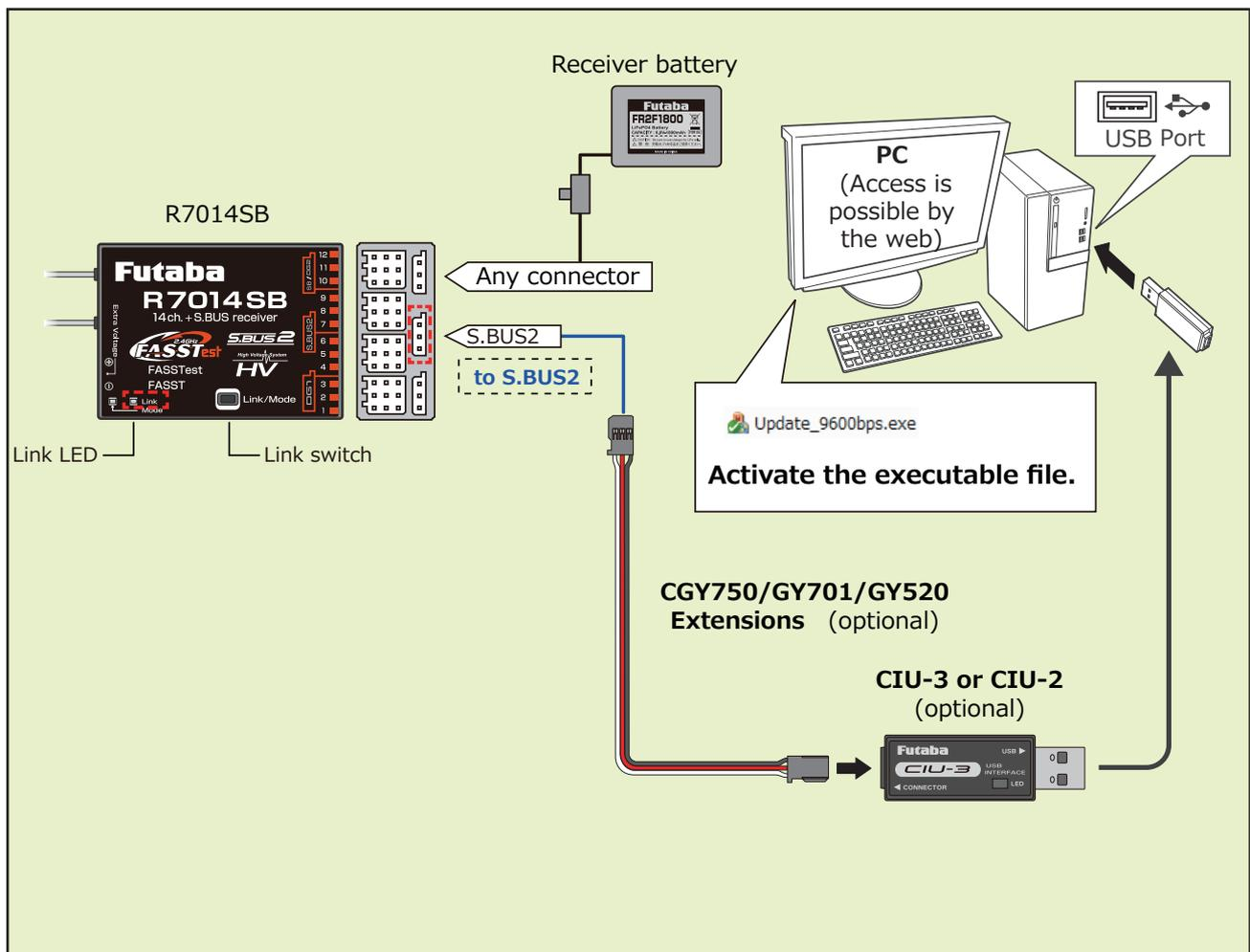
4. Turn on the receiver power while pressing down the Link switch.
