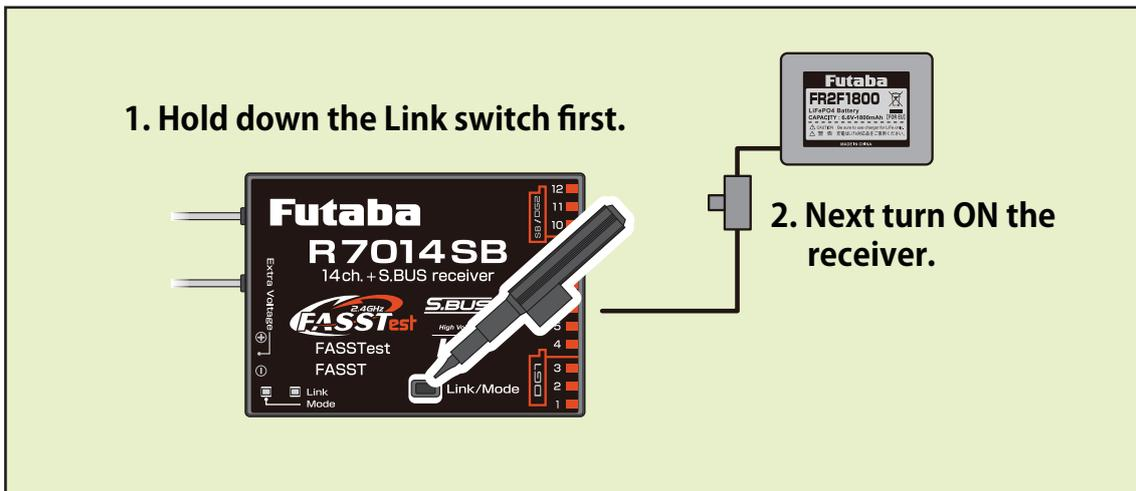
5. Once LED confirms the to "red flashing once", release the Link switch once, and re press again.
