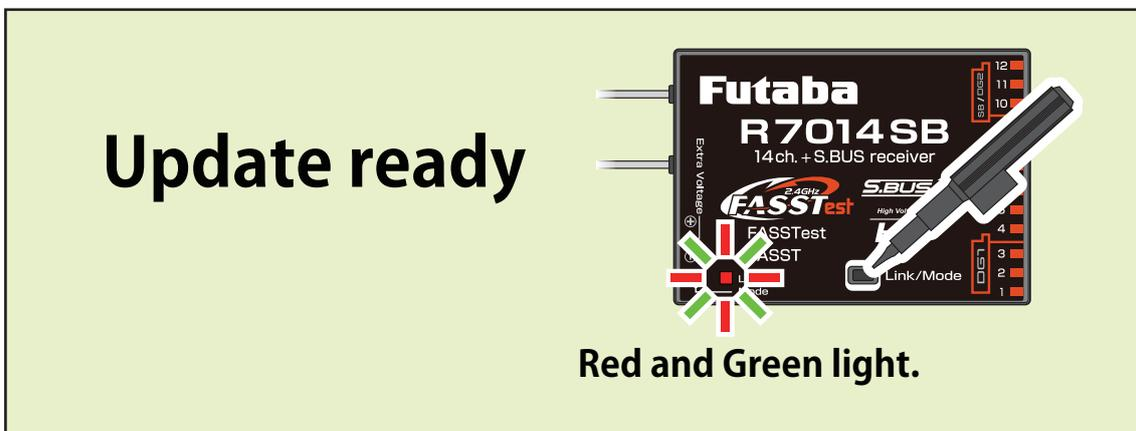
7. Operate the PC update. (The receiver should keep red and green on.)
