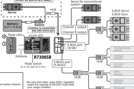
\*Never use dry batteries for the power sup-ply of the R7308SB as they may cause difficulties.
