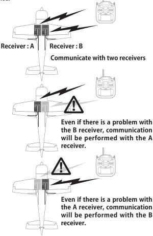
In Dual RX link mode, the SB2/RX port is for reception only, so use CH mode B, C, D, F, G mode for S.BUS output and S.BUS2 input/output.
