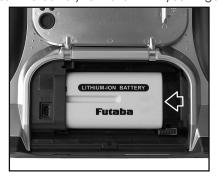
4. Close and lock the battery cover completely.
