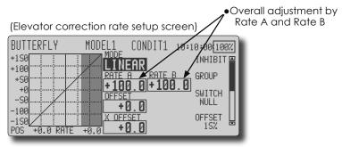
Mixing curve setting \*For a description of the curve setting method, see the description at the back of this manual.
