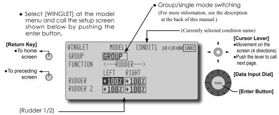
• The travel at rudder stick left and right operation can be individually set.
