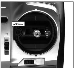
Use the attached 1.5mm hexagonal wrench to turn the screw clockwise to adjust the stick outwards, or counter-clockwise to tilt it inward.
