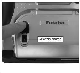
This is the connector for charging the Lithium Ion battery LT2F2200 that is installed in the transmitter. Do not use any other chargers except
