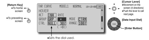
The Throttle Hover function trims the throttle near the hovering point. Normally, use it with hovering conditions. Changes in rotor speed accompanying changes in the temperature, humidity, and other flight conditions can be trimmed. Adjust the throttle so that rotor rotation is most stable. More delicate trimming is also possible by using this function along with the Hover Pitch function.
