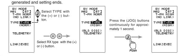
\*When using an FHSS (R603GF/R2004F, etc.) or S-FHSS(SFH) system (R2104GF, R204GF-E, etc.) receiver, after the end of setting up to here set the transmitter power switch to OFF and go to "Receivers other than T-FHSS".
