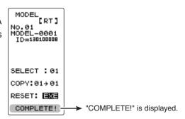
When completed, move the cursor to [RT] by the (JOG) button, and return to the MENU1 screen by pressing the (JOG) button.
