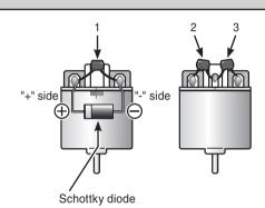
Motors with no suppressor capacitors, or inadequate suppression, may cause the receiver to malfunction. Always solder the capacitors supplied to your motor.
