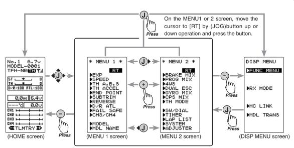
On the DISP MENU screen, move the cursor to "FUNC MENU" by (JOG) button up or down operation and press the button.
