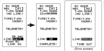
the PWR ON position. If the receiver LED lights green, linking was successful. Check for correct servo operation.
