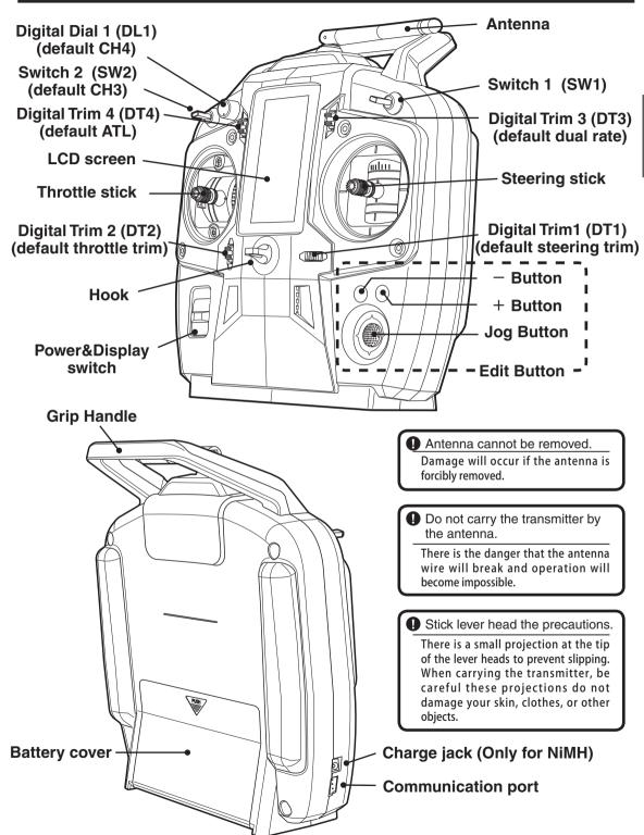
\*The switches, dial, and trimmers in the figure are shown in the initial setting position.
