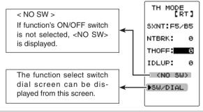
If the power switch is turned on while the idle-up switch is on, an audible alarm will be heard. Immediately set the Idle-Up switch to OFF.
