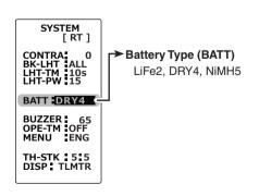
**Note:** If used with the incorrect setting, a normal low battery alarm will not be generated and the system may stop before the battery alarm is generated. The usage time may also become extremely short.
