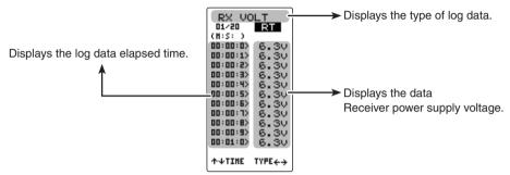
Receiver power supply voltage log.
