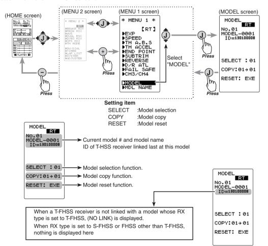
Forty model data (model data for 40 R/C cars) can be saved in the 4GRS transmitter and used when the relevant model data is called.
