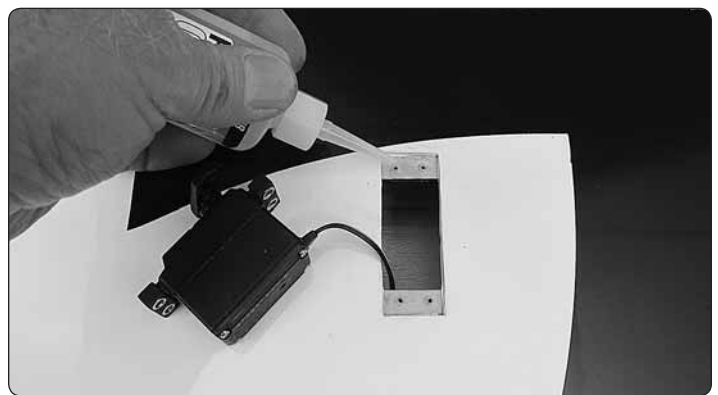
10. Apply a drop of thin CA in each hole to harden wood. After the CA has cured, reinstall the servo and servo screws.
