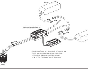
• Connect the LCD program box to the ESC as shown above, and then connect the battery to the ESC.
