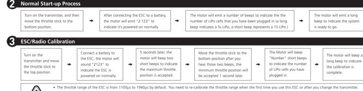
• During the ESC/Radio calibration, please set the throttle curve to NORMAL and ensure the corresponding throttle amounts to the maximum throttle endpoint and the minimum throttle endpoint on your transmitter are respectively 100% and 0%.
