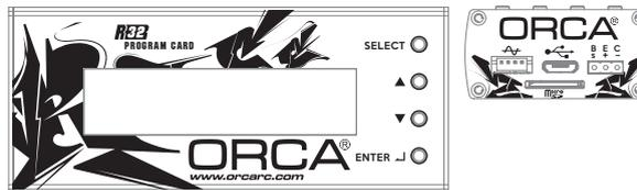
To begin, connect the battery wires to a charged battery, then connect supplied 4pin wire (200mm) to the ESC setting port (4pin port) and Program Card. Turn on the ESC and the Program Card will activate automatically. Note that the screen will show "Loading..." during initialization – indicating that the ESC is copying the current setup in the ESC to the Program Card. Once loading is completed, the screen will show "ORCA B32 Pro" and "Program". You can now begin programming your ESC.
