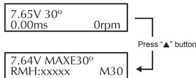
This will show the last pack of run, the min Battery Voltage, max ESC Temperature max Motor Temperature.
