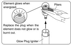
Be careful not to damage the plug threads when holding a glowplug with pliers.
