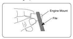
Make sure that the vehicle's engine mounting surfaces are level and in the same plane. Poor installation may cause distortion of the crankcase, bearings, etc., resulting in erratic running and loss of performance.
