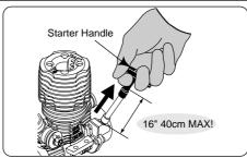
Do not attempt to disassemble the recoil starter. If you do so, the very strong spring inside will be suddenly ejected. This can be
