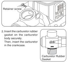
Note: In case it is hard to insert the carburetor in the crankcase, apply oil on the Thermo Insulater. Do not force it, or damage to the Thermo Insulater and/or crankcase can occur.
