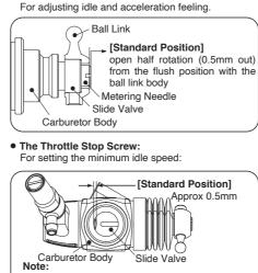
Sketch shows the carburetor reducer removed.
