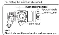
NOTE: While the Mixture Control Valve and the Metering Valve are set at the standard position when the engine leaves the factory, readjustment may be necessary, occasionally to allow for changes in fuel formula and climatic conditions Readiust the controls only when satisfactory results cannot be obtained with the standard positions following the instructions mentioned in the "CARBURETOR ADJUSTMENT" section.
