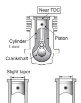
When the engine is cold. When the engine is hot.
