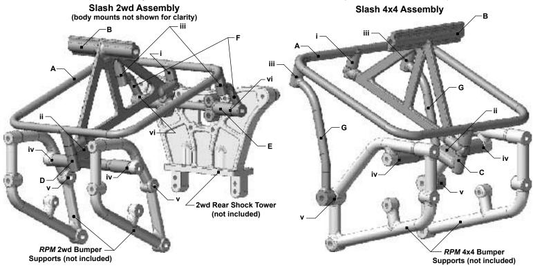
Letters (A) Support Loop, (B) Tire Mount, (C) 4x4 Rear Brace, (D) 2wd Rear Brace, (E) 2wd Shock Tower Adapter, (F) 2wd Front Braces & (G) 4x4 Front Braces.
