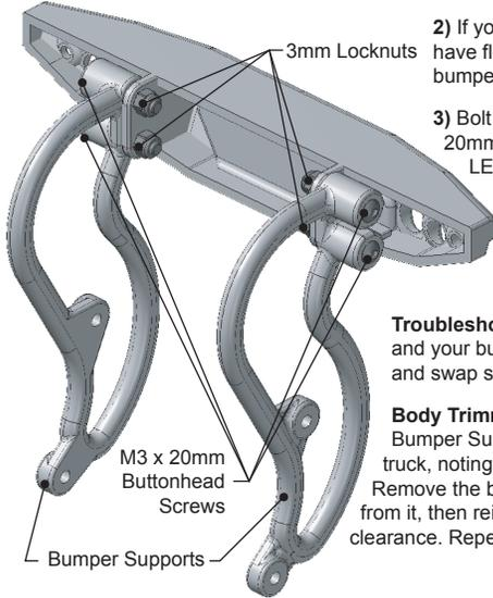
2) If you intend to install 5mm LEDs in the bumper, slip them in place in the locations shown in the Illustration above. Make sure you have flexible wire running to the LEDs since the wire must bend immediately to fit in the gap in the bumper mounts.
