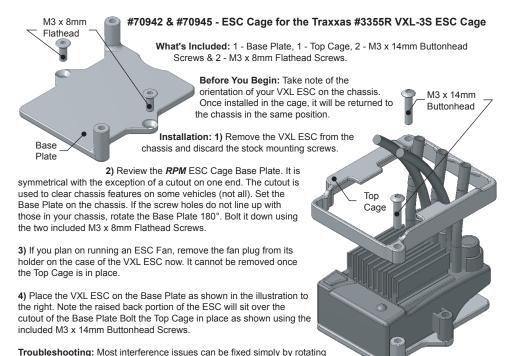
the Base Plate. Top Cage or the entire assembly by 180°.
