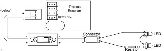
**9)** Solder your negative wire to the negative wire of the connector and solder the opposite end to the negative (cathode) of one of your LED's.
