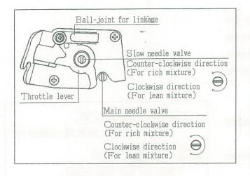
\* The target value of carburetor adjustment (throttle-valve fully closed)
