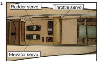
Minimum servo spec. Torque : 80 oz-in (5.8 kg-cm) @ 4.8V; 100 ozin (7.2 kg-cm) @ 6.0V
