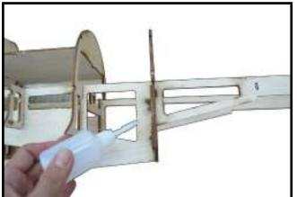
Fill Epoxy Glue around block include two layers 24.F6, F6A.
