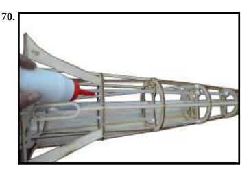
Install the plastic tube to go through all formers which have path of Fin and path of Elevator hole on each former and fill White Glue to keep fixed.
