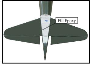
Slide the vertical stabilizer back in place. Using a triangle, check to ensure that the vertical stabilizer is aligned 90° to the horizontal stabilizer.
