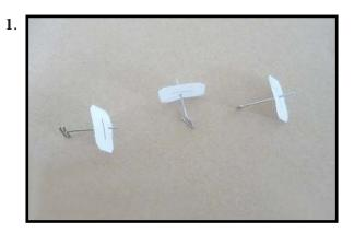
Remove each hinge from the wing panel and flap and place a T-pin in the center of each hinge. Slide each hinge into the wing panel until the T-pin is snug against the wing panel. This will help ensure an equal amount of hinge is on either side of the hinge line when the flap is mounted to the aileron.
