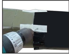
Install the muffler and muffler extension onto the engine and make the cutout in the cowl for muffler clearance. Connect the fuel and pressure lines to the carburetor, muffler and fuel filer valve. Secure the cowl to fuselage using the M3x10mm socket head screws. Putting a small length of silicon fuel tube under the head of the screw helps with vibration.
