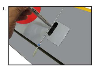
Mark the control wire where it crosses the servo arm hole.
