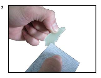
Check the fit of the control horns to the aileron and flap. They should rest flush against the control surface as shown.
