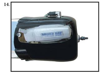
Attach the electric motor box to the firewall centered with the cross lines drawn on the electric motor box and firewall. Using M4x25mm to secure the motor box to the firewall. Please see pictures below.
