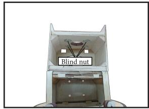
Attach the motor to the front of the electric motor box using four 4mm blind nut, four M3x15mm hex head bolts to secure the motor. Please see picture shown.
