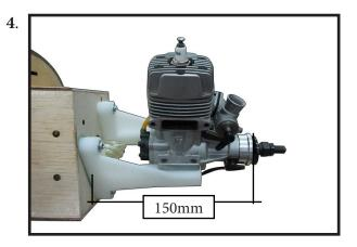
Use a pin drill and 4mm drill bit to drill a small indentation in the mount for the engine mounting screw.
