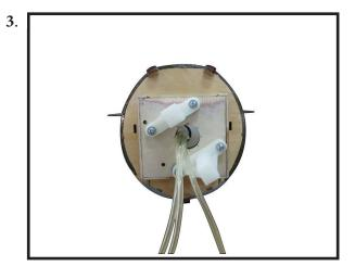
Position the engine with the drive washer (150mm) forward of the fiewall as shown.
