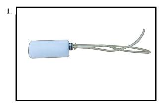
You should mark which tube is the vent and which is the fuel pickup when you attach fuel tubing to the tubes in the stopper. Once the tank is installed inside the fuselage, it may be difficult to determine which is which.
