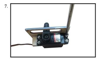
Apply 1-2 drops of thin C/A to each of the mounting tabs. Allow the C/A to cure without using accelerator.
