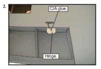
Slide the wing panel on the flap until there is only a slight gap. The hinge is now centered on the wing panel and flap. Remove the T-pins and snug the aileron against the wing panel. A gap of 1/64" or less should be maintained between the wing panel and flap.
