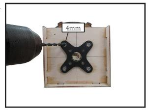
Then, use 4mm drill bit to enlarge the holes on the electric motor box.
