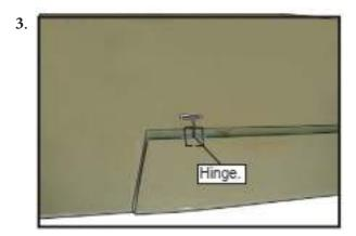
Deflect the aileron and completely saturate each hinge with thin C/A glue. The ailerons front surface should lightly contact the wing during this procedure. Ideally, when the hinges are glued in place, a 1/64" gap or less will be maintained throughout the length of the aileron to the wing panel hinge line.
