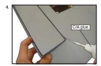
Turn the wing panel over and deflect the flap in the opposite direction from the opposite side. Apply thin C/A glue to each hinge, making sure that the C/A penetrates into both the aileron and wing panel.
