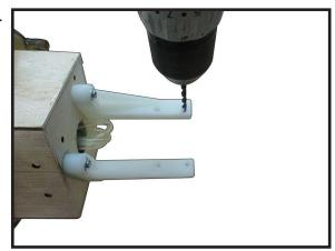
On the fie wall has the location for the throttle pusshrod tube (pre-drill).
