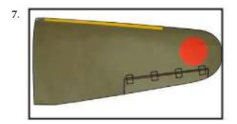
Note: Work the aileron up and down several times to "work in" the hinges and check for proper movement.
