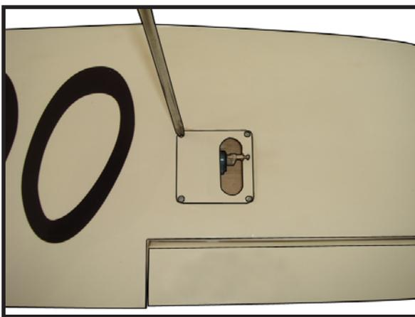
3) Set the aileron hatch in place and use a Phillips screw driver to install it with four wood screws.
