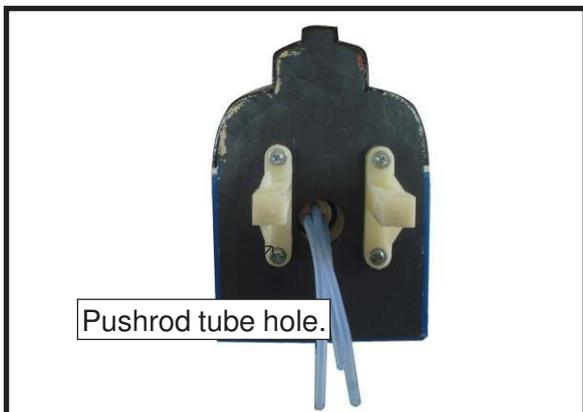
5) Slide the pushrod tube in the firewall and guide it through the fuel tank mount. Use medium C/A to glue the tube to the firewall and the fuel tank mount.
