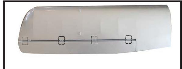
**Note:** *Work the aileron up and down several times to "work in" the hinges and check for proper movement.*
