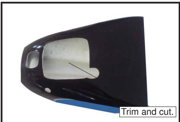
□ 2) While keeping the back edge of the cowl flush with the marks, align the front of the cowl with the crankshaft of the engine. The front of the cowl should be positioned so the crankshaft is in **nearly** the middle of the cowl opening. Use the spinner backplate as a guide. Hold the cowl firmly in place using pieces of masking tape.
