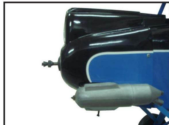
*Because of the size of the cowl, it may be necessary to use a needle valve extension for the high speed needle valve. Make this out of sufficient length 1.5mm wire and install it into the end of the needle valve. Secure the wire in place by tightening the set screw in the side of the needle valve.*
