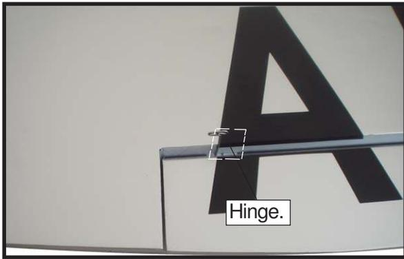
□ 4) Deflect the aileron and completely saturate each hinge with thin C/A glue. The ailerons front surface should lightly contact the wing during this procedure. Ideally, when the hinges are glued in place, a 1/64" gap or less will be maintained throughout the length of the aileron to the wing panel hinge line.
