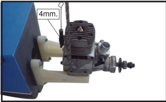
3) Use a drill to drill the four holes in the engine mount rails.
