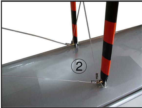
3) Begin placing tension on the wires, working from the ends that have been crimped to the ends that have not. There should be light tension on all the cables, but not enough to change the position of the wing. Once the cables have been tensioned, begin by securing the crimps where the cables pass through the tabs near the fuselage. Then secure the crimps at the cable ends. Once tensioned, use side cutters to trim the excess cable.
