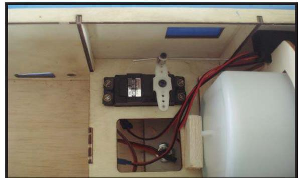
9) Move the throttle stick to the closed position and move the carburetor to closed. Use a 2.5mm hex wrench to tighten the screw that secures the throttle pushrod wire. Make sure to use threadlock on the screw so it does not vibrate loose.
