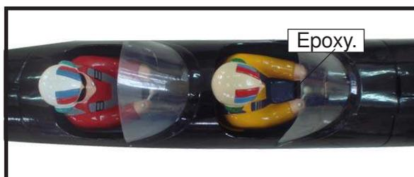
4) Position the canopy onto the fuselage. Trace around the canopy and onto the fuselage using a felt-tipped pen.
