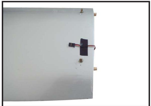
9) Set the aileron hatch in place and use a Phillips screw driver to install it with four wood screws.
