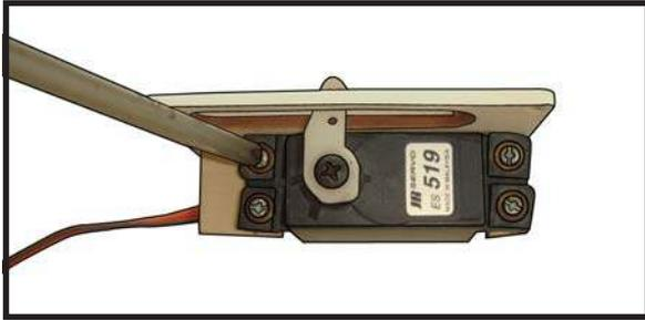
7) Apply 1-2 drops of thin C/A to each of the mounting tabs. Allow the C/A to cure without using accelerator.
