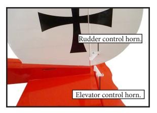
2) Elevator and rudder pushrods assembly as pictures below.
