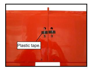
5) Reinstall the servo into the servo mount and secure the servo inplace using the wood screws provided with you radio system.
