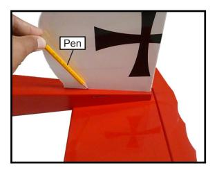
3) Remove the stabilizer. Using a modeling knife, remove the covering from below the lines you drew.
