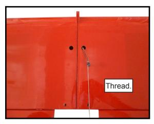
4) Tape the servo lead to the wing to prevent it from falling back into the wing.
