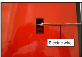
3) Attach servo lead to the aileron servo. Attach the string to the servo lead and carefully thread it though the wing. Once you have thread the lead throught the wing, remove the string so it can use for the other servo lead.
