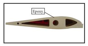
Attach the aluminum tube into wing.
