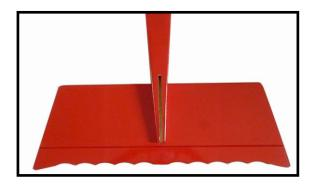
4) With the stabilizer held firmly in place, use a pen and draw lines onto the stabilizer where it and the fuselage sides meet.
