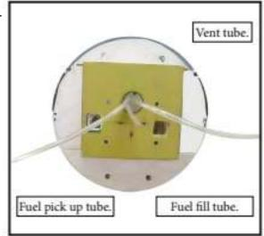
Connect the lines from the tank to the en gine and muffler. e vent line will connect to the muffler and the line from the clunk to the carburetor.
