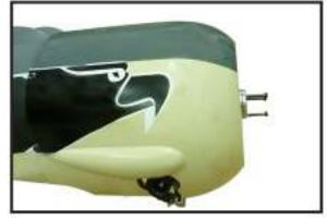
Install the muffler and muffler extension onto the engine and make the cutout in the cowl for muffler clearance. Connect the fuel and pressure lines to the carburetor, muffler and fuel filler valve. Secure the cowl to fuse lage using the M3x10mm socket head screws.
