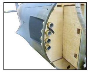
Locate the laser cut engine mounting template. Align mounting template to front of firewall.
