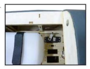
Move the throttle stick to the closed position and move the carburetor to closed.
