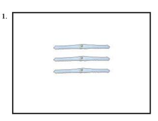
Test fit the hinges into the elevator, and then the hinges into the horizontal stabilzer. Ensure that the hinge pockets
