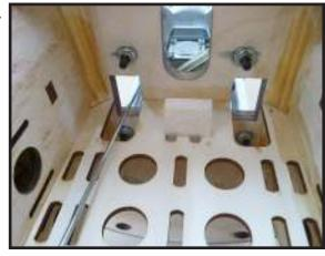
Drill a hole for the throttle pushrod.
