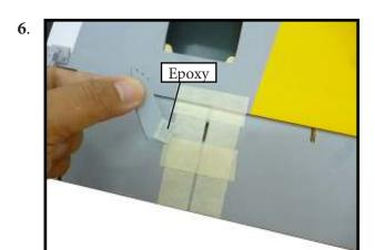
Before the epoxy fully cures, remove the tape from around the control horn. This will allow the epoxy to flow around the control horn, creating a small filet between the control horn and surface for a fiished look and secure bond.
