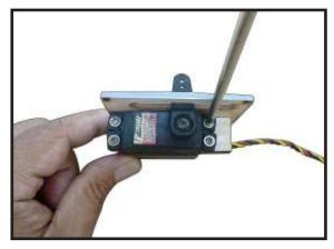
Apply 1-2 drops of thin C/A to each of the mounting tabs. Allow the C/A to cure without using accelerator.
