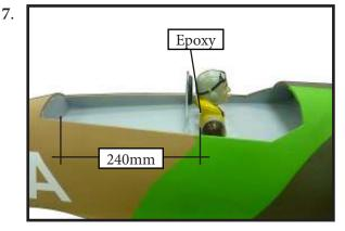
Position the canopy to the fuselage. Trace around the tree canopy and onto the fuselage with a marker. Carefully cut and remove the covering material from the fuselage where the canopy touches, exposing the bare wood. Then screw it in place.
