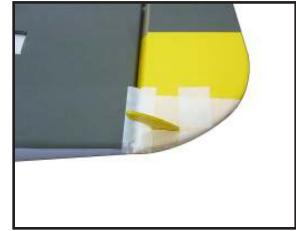
Use Epoxy to glue the Horizontal Stabilizer to the fuselage.
