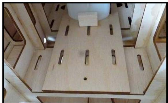
7) Use balsa block to hold in place the fuel tank with C/A glue to secure the fuel tank.
