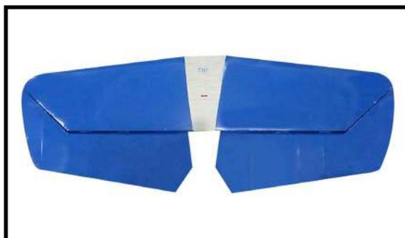
□ 7) When you are sure that everything is aligned correctly, mix up a generous amount of 30 Minute Epoxy. Apply a thin layer to the top and bottom of the stabilizer mounting area and to the stabilizer mounting platform sides in the fuselage. Slide the stabilizer in place and realign. Double check all of your measurements once more before the epoxy cures. Hold the stabilizer in place with T-pins or masking tape and remove any excess epoxy using a paper towel and rubbing alcohol.
