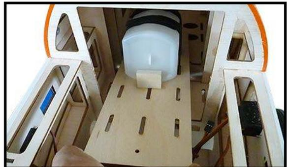
**!** You should mark which tube is the vent and which is the fuel pickup when you attach fuel tubing to the tubes in the stopper. Once the tank is installed inside the fuselage, it may be difficult to determine which is which.
