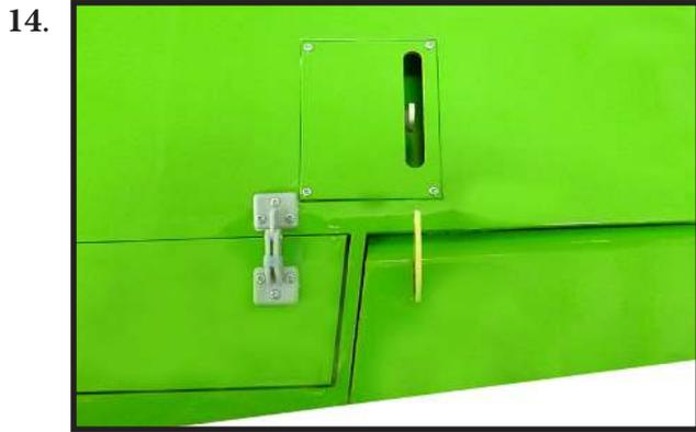
**INSTALLING THE FLAP SERVO.**
