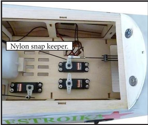
**RUDDER PUSHROD INSTALLATION.**
