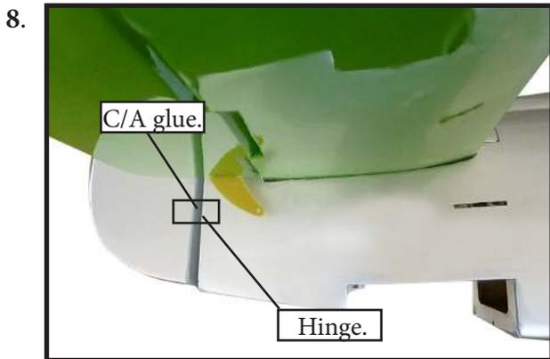
**ELEVATOR PUSHROD HORN INSTALLATION.**
