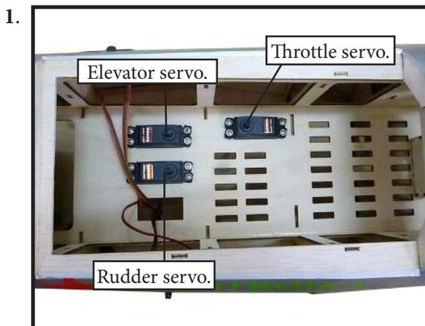
**THROTTLE SERVO ARM INSTALLATION.**
