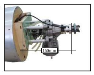
Position the engine with the drive washer (160mm) forward of the firewall.
