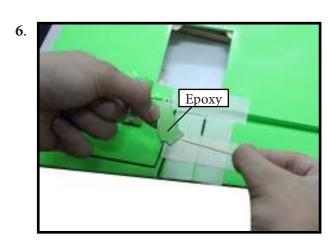
Before the epoxy fully cures, remove the tape from around the control horn. This will allow the epoxy to flow around the control horn, creating a small filet between the control horn and surface for a fished look and secure bond.
