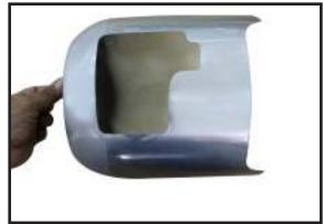
Tape the cowl to the fuselage using low-tack tape.
