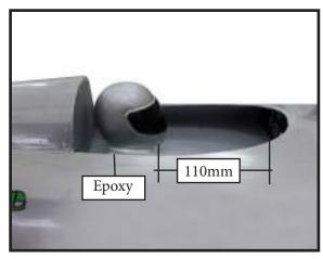
Epoxy canopy onto the fuselage. Trace around the canopy and onto the fuselage using a epoxy.
