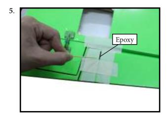
Apply epoxy to the area of the control horns that fist into the slots. Use enough epoxy so the control horns will be fully bonded to the fied surfaces.
