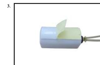
Test fit the stopper assembly into the tank. It may be necessary to remove some of the flashing around the tank opening using a modeling knife. If flashing is present, make sure none falls into the tank.
