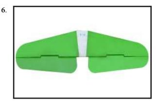
When you are sure that everything is aligned correctly, mix up a generous amount of 30 Minute Epoxy. Apply a thin layer to the top and bottom of the stabilizer mounting area and to the stabilizer mounting platform sides in the fuselage. Slide the stabilizer in place and realign. Double check all of your measurements once more before the epoxy cures. Hold the stabilizer in place with T-pins or masking tape and remove any excess epoxy using a paper towel and rubbing alcohol.
