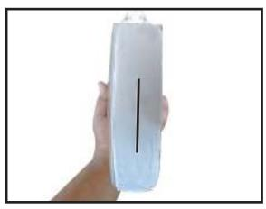
While holding the vertical stabilizer fimly in place, use a pen and draw a line on eachside of the vertical stabilizer where it meets the top of the fuselage.
