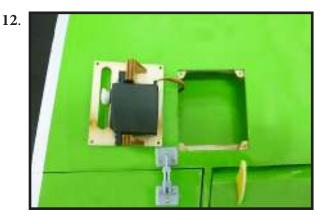
Set the aileron hatch in place and use a Phillips screw driver to install it with four wood screws.
