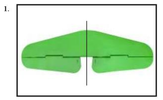
Using a modeling knife, carefully remove the covering at mounting slot of horizontal stabilizer (both side of fuselage).
