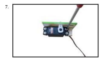
Apply 1-2 drops of thin C/A to each of the mounting tabs. Allow the C/A to cure without using accelerator.
