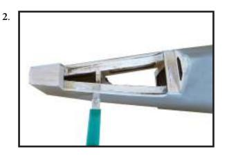
Slide the stabilizer into place in the precut slot in the rear of the fuselage. The stabilizer should be pushed firmly against the front of the slot.
