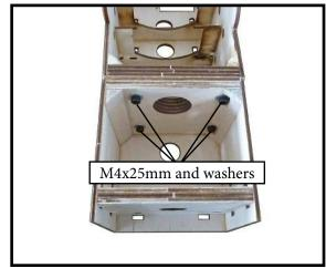
Attach the motor to the front of the electric motor box using four 4mm blind nut, four M4x25 mm hex head bolts to secure the motor. Please see picture shown.
