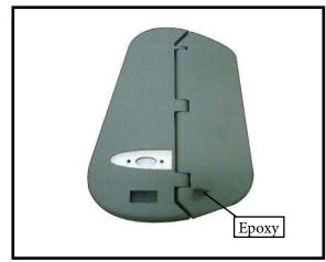
**RUDDER PUSHROD HORN INSTALLATION**
