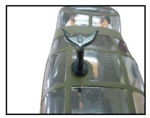
Position the plastic parts onto the canopy and fuselage and apply C/A glue and hold the plastic parts secure until the glue fully cures.
