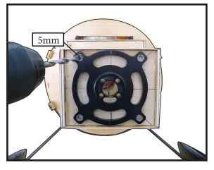
Then, use 5mm drill bit to enlarge the holes on the electric motor box.
