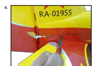
Crimp the brass tube with a crimping tool or pliers.
