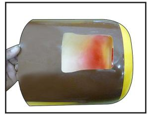
Tape the cowl to the fuselage using low-tack tape.
