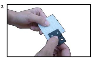
Mix a sufficient amount of 30-minute epoxy in a cup, and with a toothpick, smear epoxy in the hinge pockets of the wing panel and aileron. Slowly and carefully, insert each hinge into the wing panel. Partially remove and reinstall the hinge to ensure that you've completely coated it with glue. Clean up any excess epoxy with isopropyl alcohol, and tape the aileron in place to cure. **YAK 54**
