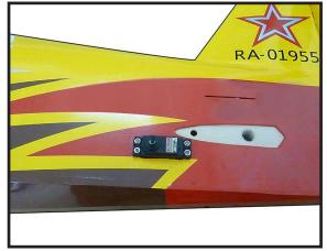
**Minimum servo spec. Torque**: 333.00 oz-in (23.98 kg-cm) @ 6.0V; oz-in (29.02 kg-cm) @ 7.4V
