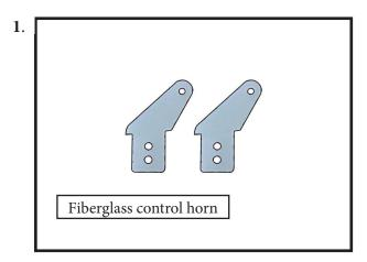
Prepare the aileron control horns by sanding the section that extends into the control surface with medium grit sand paper. Use isopropyl alcohol and a paper towel to remove any excess debris from the control horn.
