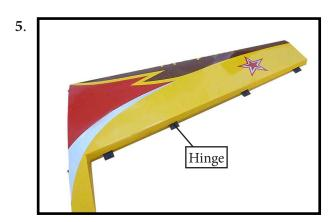
Press the aileron and wing together such that less than a 1/64" hinge line gap exists between the aileron and wing. The bevels should virtually touch. Use a paper towel and rubbing alcohol to wipe away any visible epoxy around the hinges.
