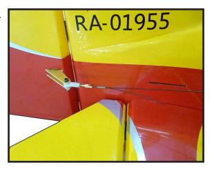
Loop the cable back through the brass swage tube and tighten the second loop through the brass swage tube as shown.
