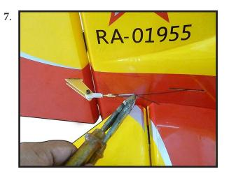
Cut off excess cable as shown.
