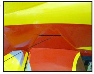
Thread cable through brass swage tube.
